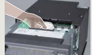
Easy access to the thermal head for cleaning.
